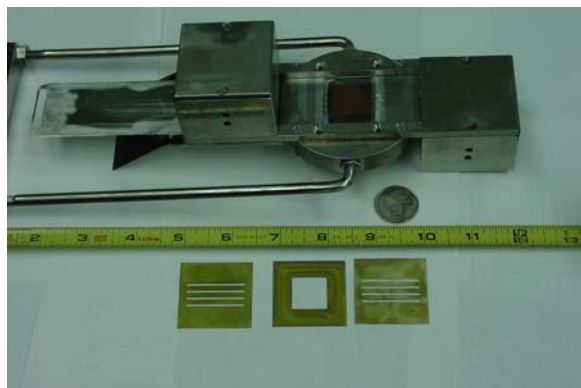
Figure 2. In-situ mask changing unit, shown with masks.
