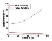
Fig. 2: Empirical mean of the epipolar distances. True target matching produces low epipolar distances.
